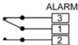
Relay shown in non-faulted condition
